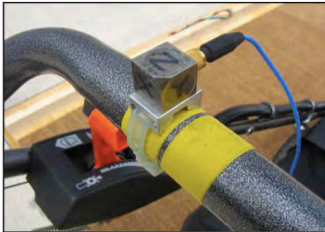
Figure 3 Aluminium block positioned using the cable tie system
