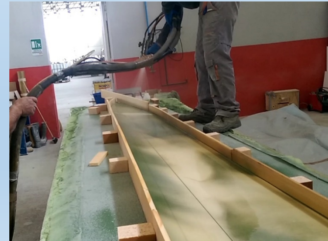
Spray polyurethane plug
